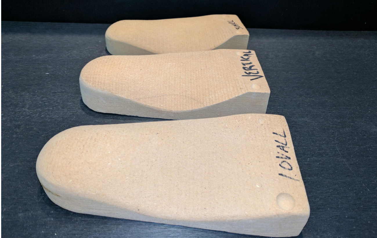
Fig. 4, Positive Casts generated through CAD/CAM technology
